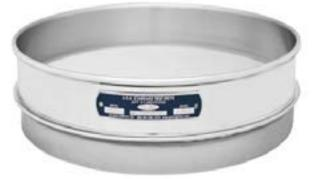
The frame of a 12" half height stainless-stainless sieve is 15/8" above the mesh. All of the 12" half height sieves come with a certificate of compliance and meet the ASTM E11 requirements. The overall height of the half height sieve is 2 5/8in and stacked height is  $1\frac{3}{4}$  in.
