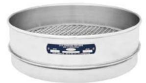
A 12" intermediate height stainless-stainless sieves frame is 2" above the mesh. All intermediate height sieves meet the ASTM E11 requirements and comes with a certification of compliance. Its overall height is 3" and its stacked height is 2 1/8in.
