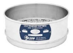
An 8" full height stainless-stainless sieve has a frame height that is 2" above the mesh. Each full height sieve meets the requirements of the ASTM E11 and include a certificate of compliance. The overall height is 2 5/8in and stacked height is 2 1/8in.
