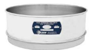
A 12" full height stainless-stainless sieve comes with a certificate of compliance and meet the ASTM E11 requirements. The frame of the full height sieve is 3" above the mesh. The overall height is 4 ¼ in and stacked height is 3 3/8 in.
