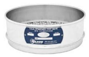
The 8" half height stainless-stainless sieve meets the requirements of ASTM E11 and includes a certificate of compliance. The frame height of the 8" half height sieve is 1" above the mesh. The overall height is 1 5/8in and stacked height is 1 1/8in.
