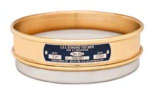
The 8" half height brass-stainless sieve meets the requirements of ASTM E11 and includes a certificate of compliance. The frame height of the 8" half height sieve is 1" above the mesh. The overall height is 1-5/8in and stacked height is 1-1/8in.
