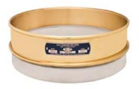
The frame of a 12" half height brass-stainless sieve is 2" above the mesh. All of the 12" half height sieves come with a certificate of compliance and meet the ASTM E11 requirements. The overall height of the half height sieve is 2 5/8in and stacked height is 1 % in.
