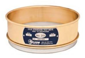
An 8" full height brass-stainless sieve has a frame height that is 2" above the mesh. Each full height sieve meets the requirements of the ASTM E11 and include a certificate of compliance. The overall height is 2-5/8in and stacked height is 2-1/8in.
