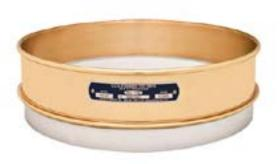
A 12" intermediate height brass-stainless sieve frame is 1-5/8in above the mesh. All intermediate height sieves meet the ASTM E11 requirements and comes with a certification of compliance. Its overall height is 3" and has a stacked height of 2-1/8in.
