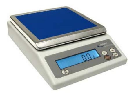
The PD Series Precision balance comes with a CalQuick single button calibration function, making calibration simple, as well as ensuring the balance is being calibrated often during use. The large stainless steel pan allows for easy weighing of large objects, while the balance also includes a below balance for more bulky items and density calculations. PD Series are great for portability with its battery operation, the balance can be used in various locations without access to 120 Volt power.
