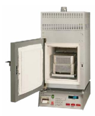
NCAT Binder Ignition ovens automatically determines asphalt content of paving mixtures. The oven is environmentally-friendly and cost-effective for the accurate determination of asphalt content. The ignition method reduces testing time compared to solvent testing methods. In addition it features an internal electronic balance that automatically monitors sample weight throughout the ignition process and determines endpoint.
