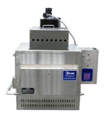
The Binder Ignition oven is a simple, manually operated oven that determines asphalt content. Samples are processed in 30-45 minutes where samples larger up to 3,000g or more require longer times. Process times are comparable to automatic-weighing units and results equal or exceed the accuracy of automated systems.
