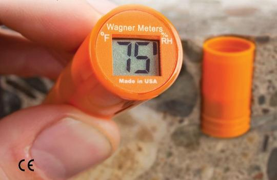
he Rapid RH® moisture testing system should be used on any project where moisture-sensitive floor coverings or coatings are to be applied over concrete slabs. Owners, general contractors, flooring contractors/installers and testing companies need to be sure the tests they perform are accurate, repeatable and available to all who need to know the current moisture condition of concrete slabs.
