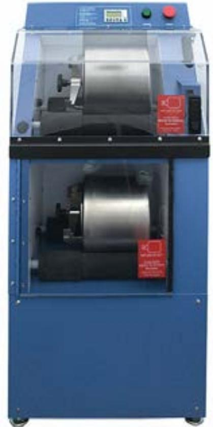
The Micro-Deval Apparatus is a second generation, state-of-the-art machine. The machine has an electronic controller with an optical sensing system that accurately tracks test time, total revolutions and rpm of jars. The Micro-Deval is a two-tier unit with a sturdy steel frame. Each tier carries one stainless steel 5L jar.
