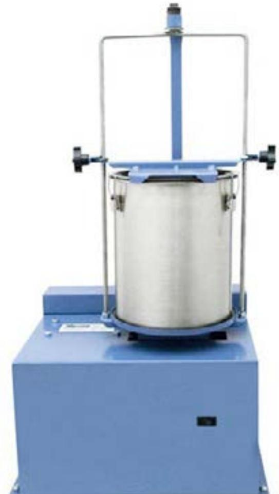
The Durability Index measures the relative resistance of aggregates. It produces clay-like fines when mechanically agitated in a special washing vessel. The resulting fines material is evaluated using the sand equivalent apparatus that is sold separately. The machine runs at 285cpm. It can also be used as a sieve shaker for up to six full-height 8in or 200mm diameter sieves and pan. Holes are provided on the unit, giving the option for securing flanges to the floor or a bench.
